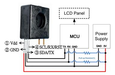
(1) DWCS **TX/RX** pin is **open drain**, and pull-up resistor must be used. If the MCU **TX/RX** pin has been internally pulled up, the resistor can be removed.
