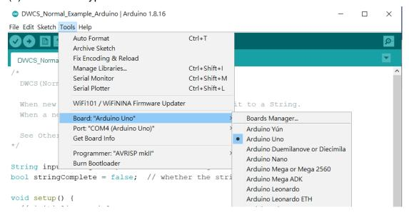
(2). Check the port of Arduino is connected and selected correctly.
