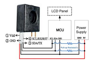
(1) DWCS **SDA/SCL** pin is **open drain**, and pull-up resistor must be used. If the MCU **SDA/SCL** pin has been internally pulled up, the resistor can be removed.
